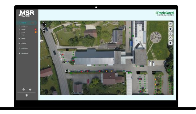
The system's background layout is customisable and can be an aerial image, a CAD drawing, a 3D drawing etc. .
